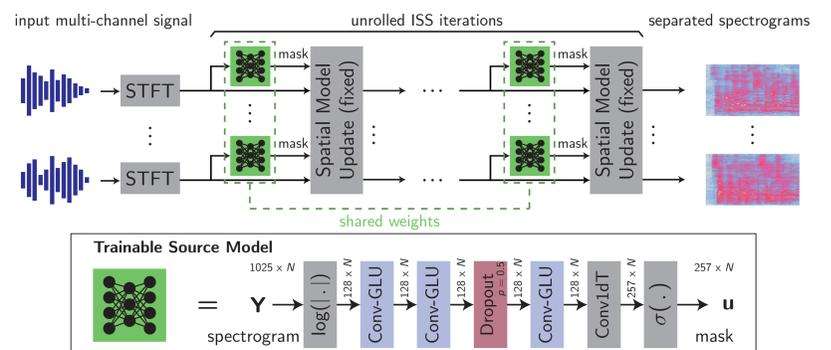
We learn the source model end-to-end from the SELD dataset using a spatial loss [4]. The model has 2.4 M parameters.
